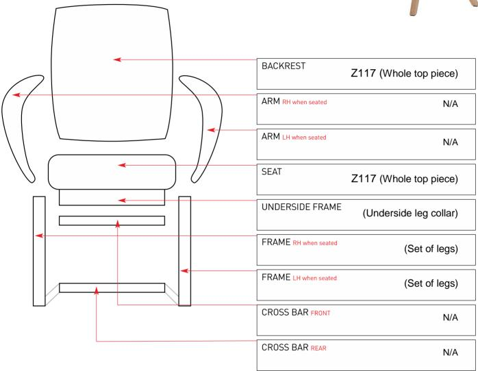
FIXINGS M6X30 SCREW x8, M6x14 SCREW x4, RECIPIENT SCREW M6\*15 x8, M6 WASHER x8, ALLEN KEY,
